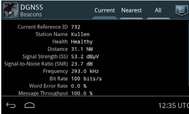
Figure 18: DGNSS Beacons - Current beacon
