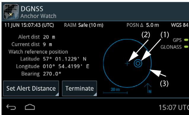
Figure 23: Anchor Watch - vessel and watch reference position
