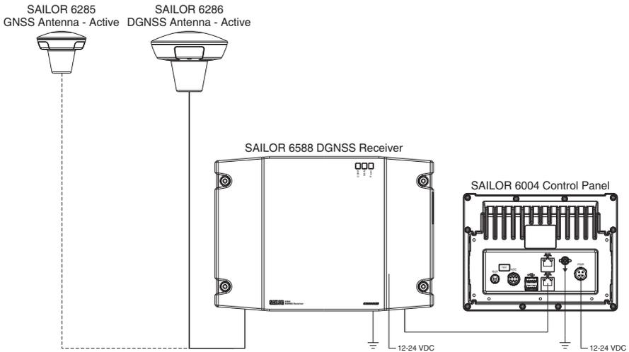
Figure 1: System configuration
