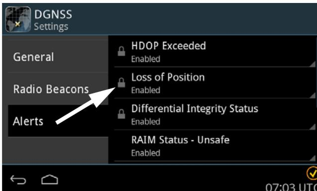
Figure 30: Password protection – example
