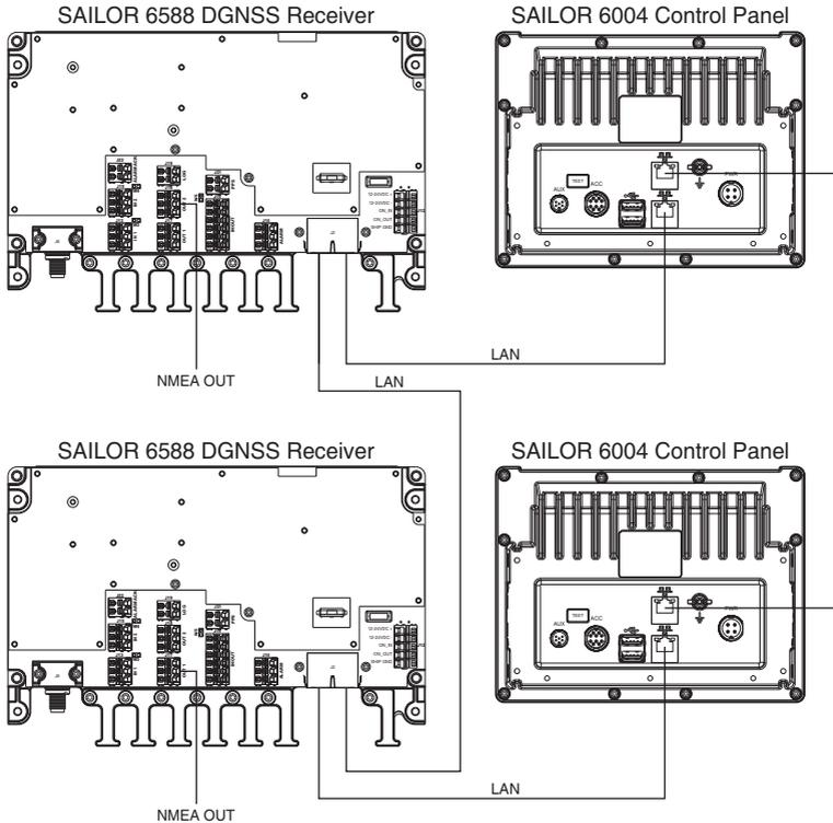
Figure 32: Multiple receivers in one system
