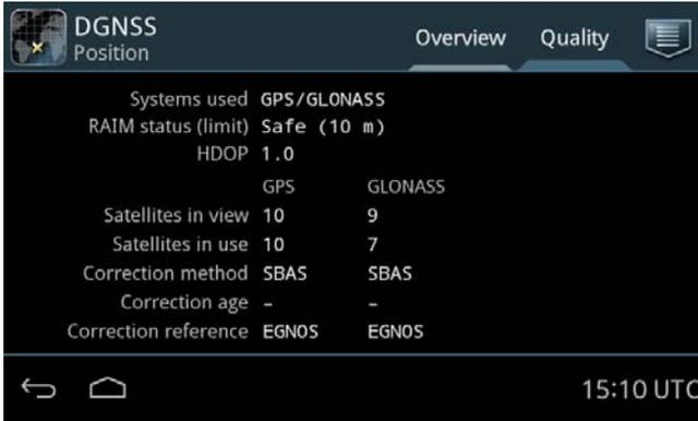
Figure 17: Using SBAS corrections
